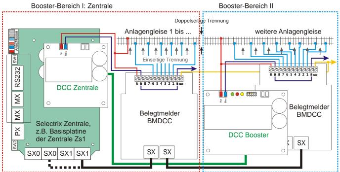
Remark: For large model railway layouts an additional ground wiring of the SX bus using the GND terminal (yellow) is recommended.
